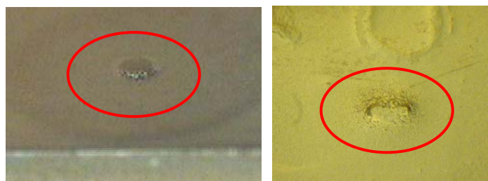
Figure 8.1-8 — Solid protrusions in substrate areas
