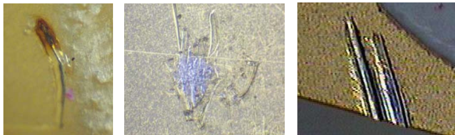
Figure 8.1-5 — Exposed base metal on packages
