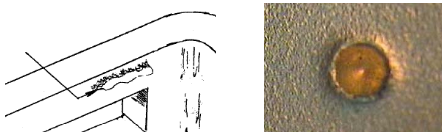
Figure 8.1-12 — Solid protrusions in general package areas
