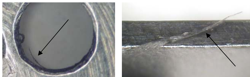
Figure 8.1-6 — Hanging protrusions
