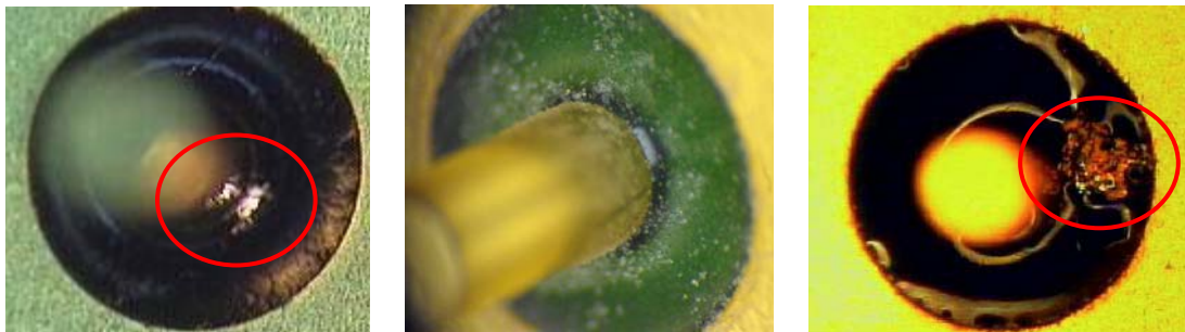
Figure 5.4-1 — Embedded foreign material in insulators
