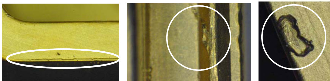
Figure 8.1-7 — Solid protrusions in critical seal areas
