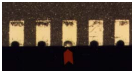
Figure 11.2-1 — A protrusion on a contact pad (Photo used with written permission of Chipworks, Inc.)
