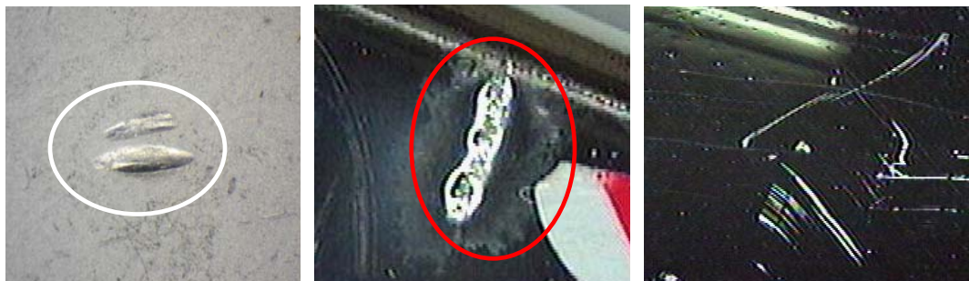
Figure 9.1-3 — Nicks, pits, voids, and indentations on general cover areas
