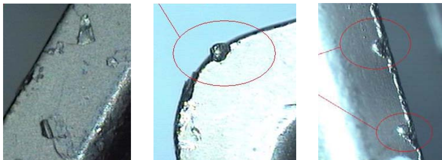
Figure 9.1-2 — Nicks, pits, voids, and indentations on cover critical seal areas
