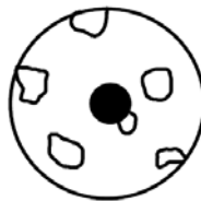
Figure 5.1-4 — Multiple subsurface bubbles
